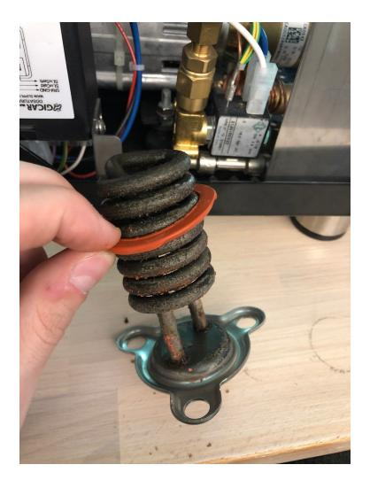
Since this is one of our test machines at the office, this picture is just for demonstration. But you can see the orange debris left from the gasket on the heating element itself. That is the reference debris that you would want to clean off if you are reusing your heating element.
