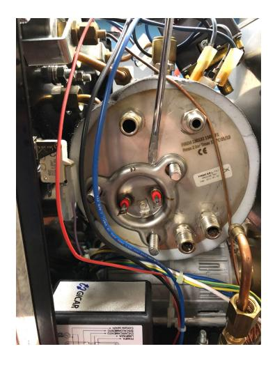
Slide the element out, you should now be looking at an open boiler:
