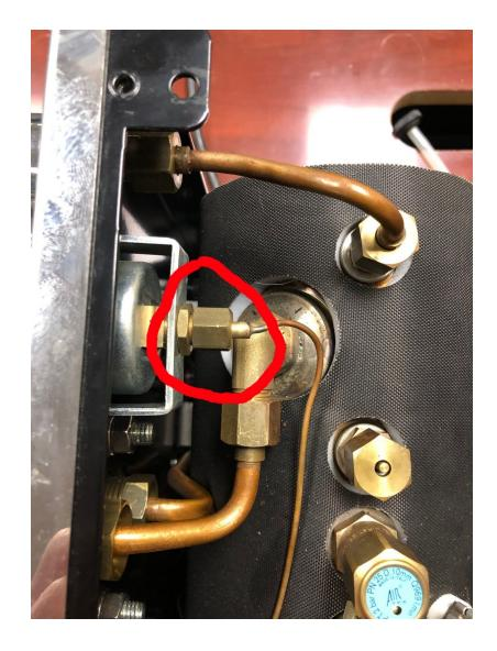
This should give you enough freedom to move the line out of the way so you can access the nut we referenced in the example earlier. To undo this nut, you will need your 12mm wrench.
