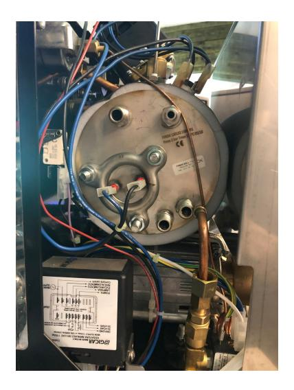
From here, label or take a picture of where you're electrical leads go before removing, and you're going to just pull the two electrical leads off of the heating element bottom/boiler. Once you've pulled those off, it's time to remove the heating element. All you need to do is remove the 3 bolts that hold it in circled below. They take the 13mm wrench:
