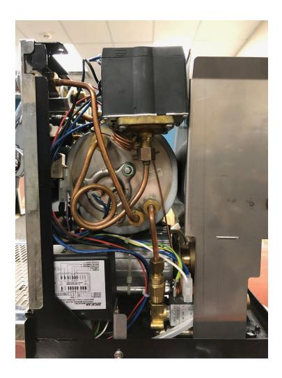
Depending on which machine you have, you may not be removing all of the same hard-lines. Machines like the Profitec Pro 500PID do not have as many hard-lines as the other machines in the line up, making them slightly less intensive to take apart.
