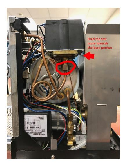
Once that is removed and set aside, you'll want to remove the hard-line that it was connected to. While you're in there, I would also recommend removing the other end of the steam pressure gauge as well. It can get in the way of undoing nuts later on. You will use your 17mm wrench to remove this line, and the 12mm again to remove the other end of the steam gauge line.
