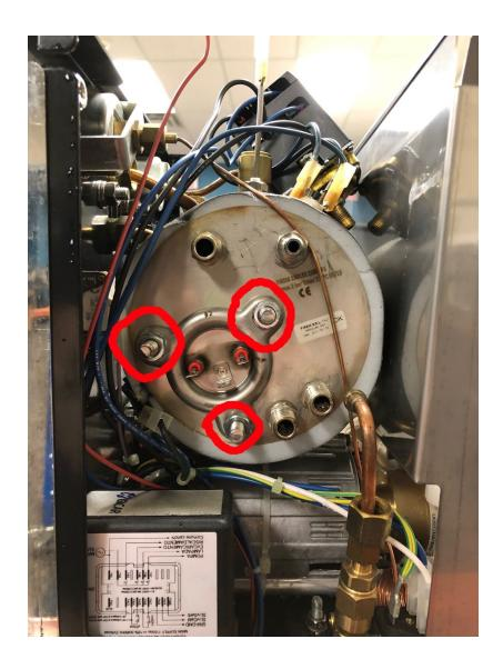
Once you've got those removed, the heating element should be able to be slid out. You may need to work it loose at first with something like a flat head. Gently wedge the flat head in between the heating element flange and the boiler, and lightly wiggle around - similarly to say, opening a paint can:
