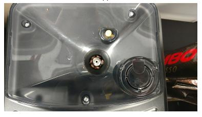
4. The sensor is a small white cylinder near the bypass doser, ensure that it is in place in the bracket with the wire facing down and the non connected end facing up. If applying a magnet directly to this sensor doesn't resolve the error, the sensor is likely damaged or disconnected and the machine will require a repair.
