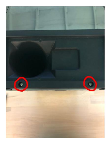
Once these have been removed, the lid from the Classic should be able to be lifted off. The black reservoir portion and the metal portion are 1 piece. Next, locate the solenoid valve. It is the assembly with the black box that is bolted to the back of your boiler:
