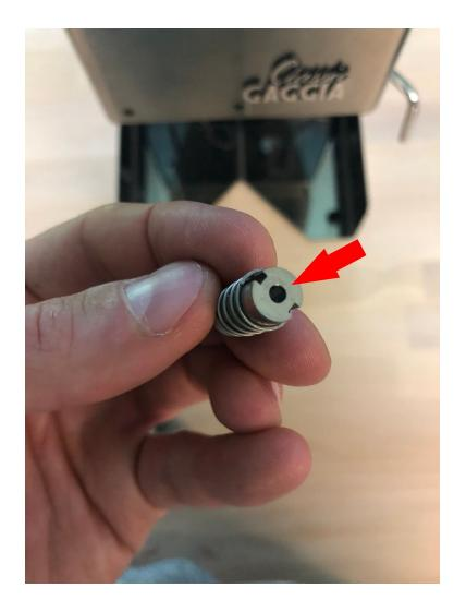
The most important piece is the lower assembly. This piece is where the clogging and blocking typically occurs. You will want to remove the o-rings, and soak this piece for 30 min - 1 hour in hot water or descaler and water, and then have compressed air blown through the various holes on it. The compressed air is an important part, make sure that you are able to do this. If you don't have an air compressor, a tire filler at a gas station will work.
