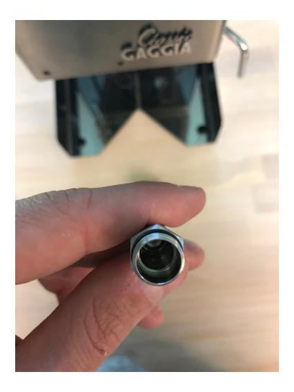
Check over the internal valve piece and make sure there is no build up on that either. There's two little black caps at either end of the valve piece. You can get a paper clip or a pen cap and push on these. Make sure they have some movement to them; they don't move much.
