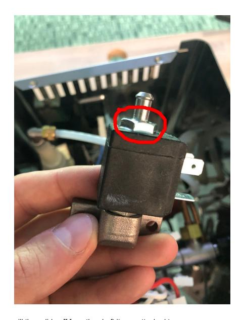
The black box will then slide off from the shaft it was attached to:
