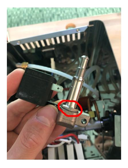
From here, you will use your 14mm wrench to undo the nut at the bottom of the shaft in the picture above. Do not force this piece off if you can't get it off. It does/can require some force to break free, but scale can line the inside of it and solidify, which can cause the threading to crack if too much force is applied. Inside the shaft is a valve piece covered by a spring. You should now have it completely disassembled, and all the pieces apart:
