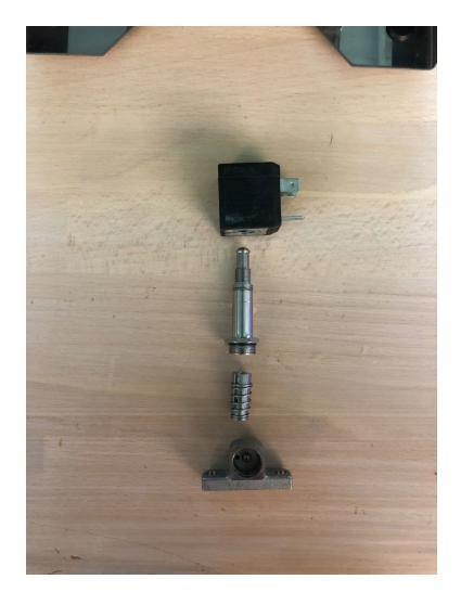
For cleaning the solenoid, check over the shaft portion and make sure there's no build up inside of it:
