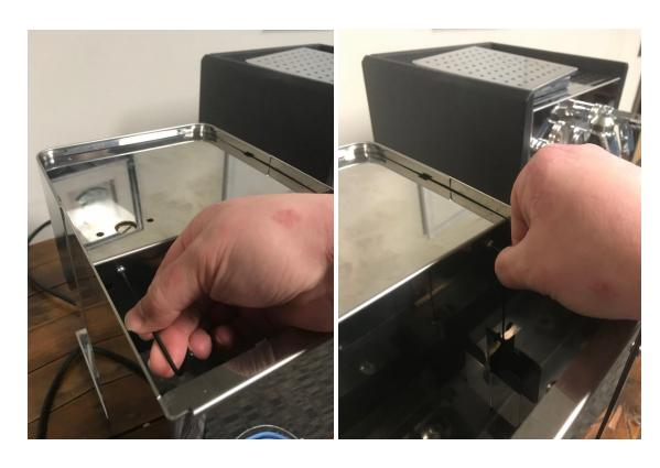
4. Once the panel is removed, you will be able to press the small grey button between the two connectors on the high limit to reset it.
