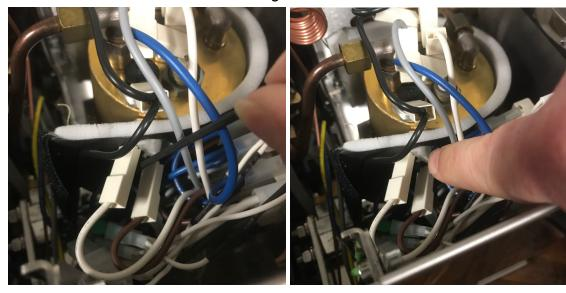
5. After pressing the button in a few times, the switch should be reset. You can replace the panel, screws, and water reservoir and plug the machine back in. Power the machine on and your machine should heat. If the machine still does not heat, the high limit may have failed and may need replaced. This would be part ECM-C199901549.
