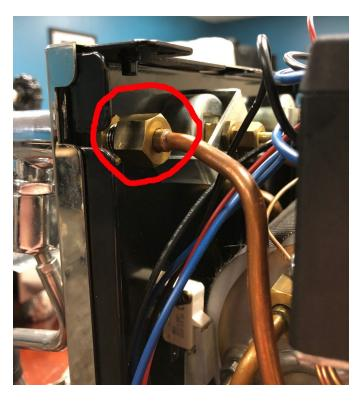
When you follow this line back to the other side to remove it, you'll run into the nut we mentioned earlier. You shouldn't have to remove the whole line, just undo the top nut with your 17mm wrench so you can gain access to the other side of the hot water valve hard-line.
