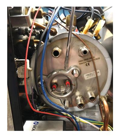
Slide the element out, you should now be looking at an open boiler.
