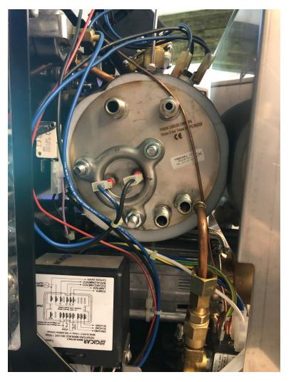
From here, label or take a picture of where your electrical leads go before removing them, pull the two electrical leads off of the heating element bottom/boiler. Once you've pulled those off, it's time to remove the heating element. All you need to do is remove the 3 bolts that hold it in (circled below). Use the 13mm wrench.
