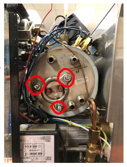
Once you've got those removed, the heating element should be able to slide out. You may need to work it loose at first with a flat head or something similar. Gently wedge the flat head in between the heating element flange and the boiler, and lightly wiggle around - like opening a paint can.
