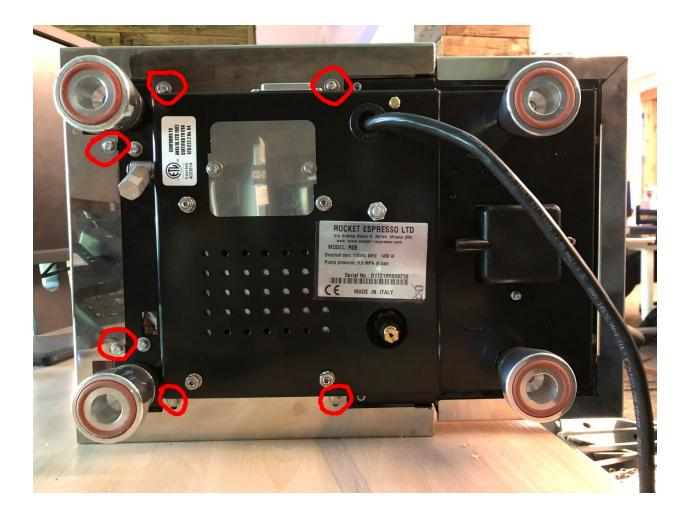
Once you've gotten those removed, you will need to remove the inverse screws. They are screws face inwards, towards the inside of the machine. There are 2 in the back left and right corners, and 2 in the front left or right corners. The will most likely require small micro turns to undo them. I would **not recommend** fully removing these, as they required a lot of small turns just to loosen them. You will use your 7mm wrench on these. Undo them just enough for the panels to come apart.
