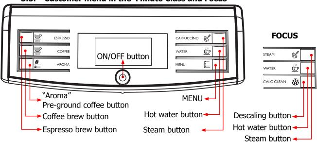
This machine is equipped with a colour-coded system to make your understanding of the display signals easier.
