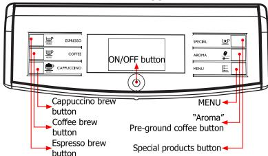
This machine is equipped with a colour-coded system to make your understanding of the display signals easier.
