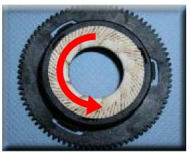
Turn the grinder blades clockwise out of the support. The bayonet connections can be accessed from the rear.
