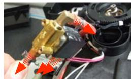
Disconnect all electrical and water circuit connections
