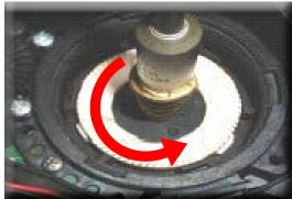
Turn the grinder blades anticlockwise out of the support.
