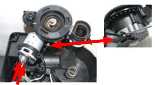
Raise the coffee grinder and remove the connections.
