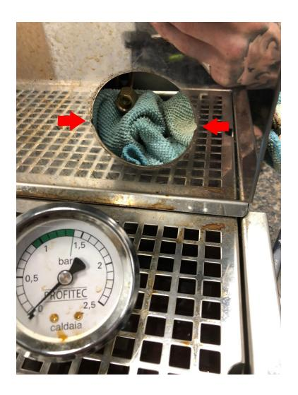
Put your new gauge back in through the front of the machine. When putting everything back on, you will want to line up the gauge so it's straight, and will need to brace the metal square with your preferred gripping tool again when tightening down the 13mm nut to make sure the gauge doesn't spin. You should now have your gauge installed, and should be up and going!
