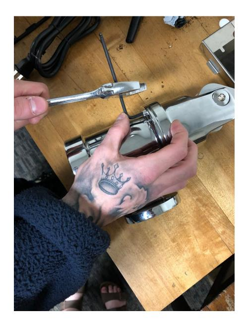
You do not need to apply excessive force when shocking. Just continue to make solid, firm taps on the allen wrench and they will come loose. Once all 4 allen screws are off, the two halves just pull apart from each other. You will have to twist and pull a little, they will be sealed together quite well. Once you get them apart, we're going to focus on the top half first with the plunger, as this is where most maintenance will occur:
