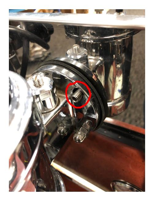
The lugs do not need to be removed, you should be able to remove the group, with the dip tube attached, from the machine in one piece. If you're working on an older machine, one of the seals we recommend having on hand is between the group, and the front panel. If this gasket is older, it very well may crumble/break apart as you remove the group:
