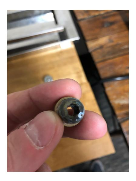
This can unscrew and come out. It requires a 6mm allen wrench. In the picture, you can see the other hole off to the left, that the water will eventually pass through to flood the group. Once out, it will just be an open cavity. You can check the piece itself for buildup, the cavity for buildup, as well as the outlet hole to the group.
