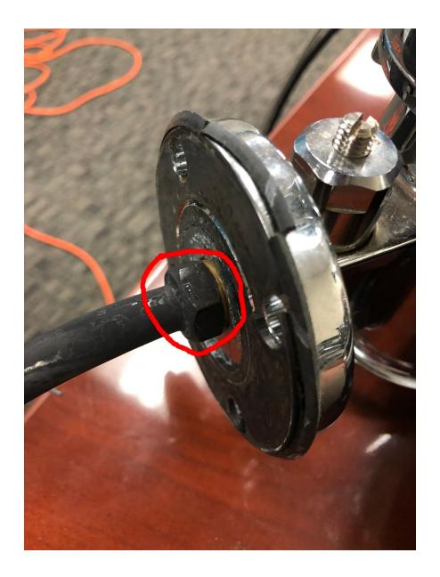
Once the dip tube has been removed, you will want to look it over for any scale buildup. If you do happen to see some buildup, you can soak it in a mixture of water and descaler, then scrub it down with a synthetic/light bristled brush to knock any stuck buildup off.
