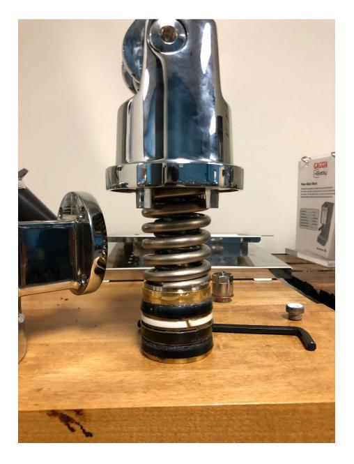
There are x4 gaskets that seal the group head to make sure water stays in the flood chamber. 3 rubber ones, and 1 teflon one. The teflon one is supposed to be cut, as teflon does not stretch. When you're replacing these seals, it's important to take note of how they go on. They do not all go on facing the same way:
