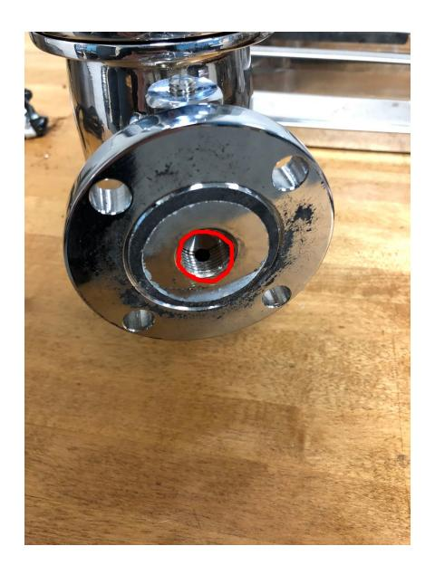
The water enters the group here, and then takes an upward path to the flood control. You will want to check this hole for buildup, and clean any out that is readily visible.
