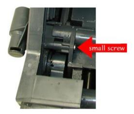
Remove the boiler connection, by pulling straight out. Set the boiler connection aside. The center section will be loose.
