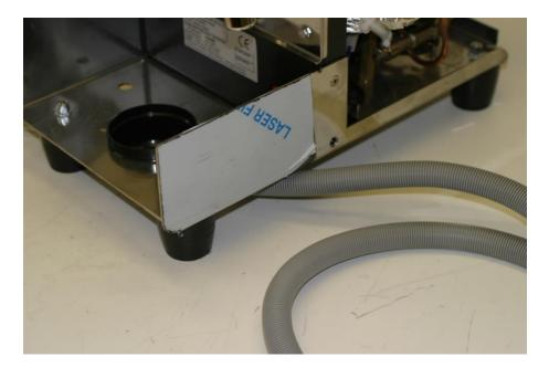
Note: Drill a  $\frac{1}{4}$ " hole in the existing drain pan.
