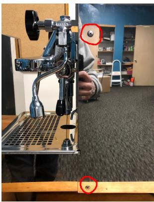
Once those have been removed, the whole housing should drop off as one assembly:
