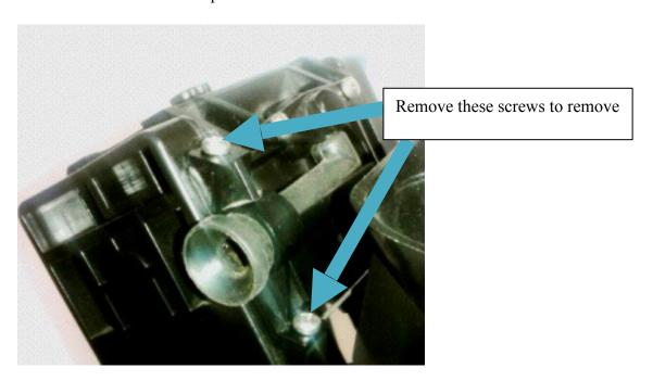
It is located near the top of the brew group. The rubber outlet tube is black and resembles the end of a trumpet. The Phillips screws are located on either side of the "trumpet" end. The opposite end of the rubber tube has a 90 degree elbow bend on it and is attached the top of the brew unit.
