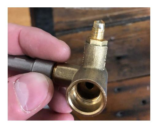
If your machine has this, do not remove it. It is needed for the silicone tubing you are removing to seal onto the nipple fitting appropriately.
