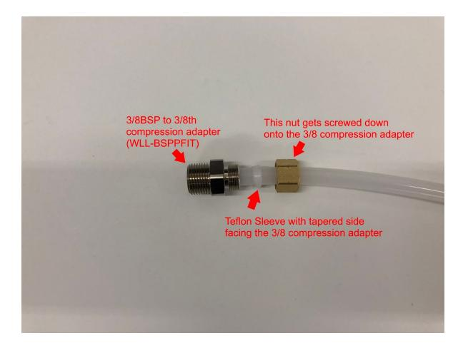
Make sure not to over tighten the nut onto the adapter.
